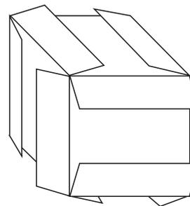
Two (unpaneled) cubes can be locked together along a face by making the folded flaps grip into each other. This allows you to build structures with these cubes.
